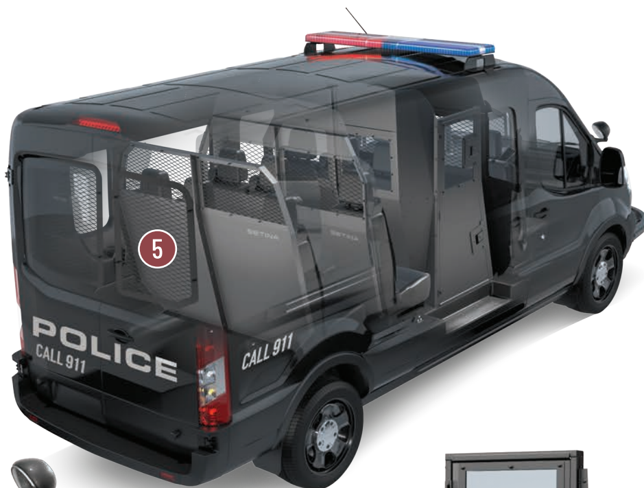
4 Enhanced Security Transport Cell Door Lockable high-security panel latch
