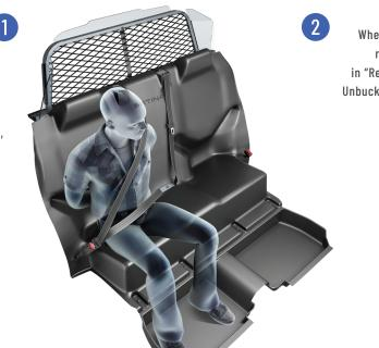
Setina's "SmartBelt" System When the belt is Buckled, the seat belt retractor is "Electronically Locked" in "Retract-Only" Mode. When the belt is Unbuckled, the "Warning Light Activates".
