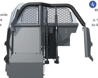
When the belt is Buckled, the seat belt retractor is Electronically Locked in "Retract-Only" Mode. When the belt is Un-Buckled, the warning Light Activates.
