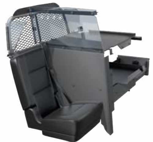
Single prisoner seating with polycarbonate And steel barrier. Barrier may vary with vehicle type. (MAX for utility shown)
